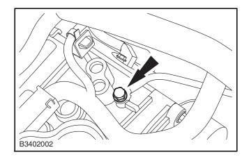
**17.** Disconnect connector between transmission wiring harness and engine compartment wiring harness.
