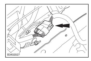
**18.** Disconnect the TCU control unit wiring harness connectors.
