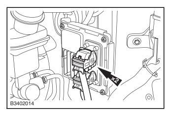
**19.** Loosen the heating inlet and outlet pipe clamps and disconnect the heating inlet and outlet pipes.
